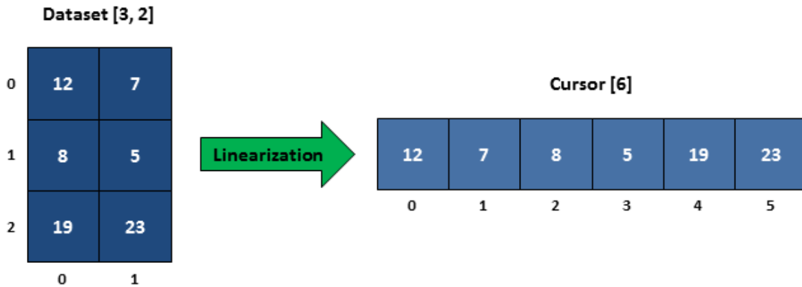
Figure 4.1 – Linearization of a two dimensional dataset into a (one dimensional) cursor
